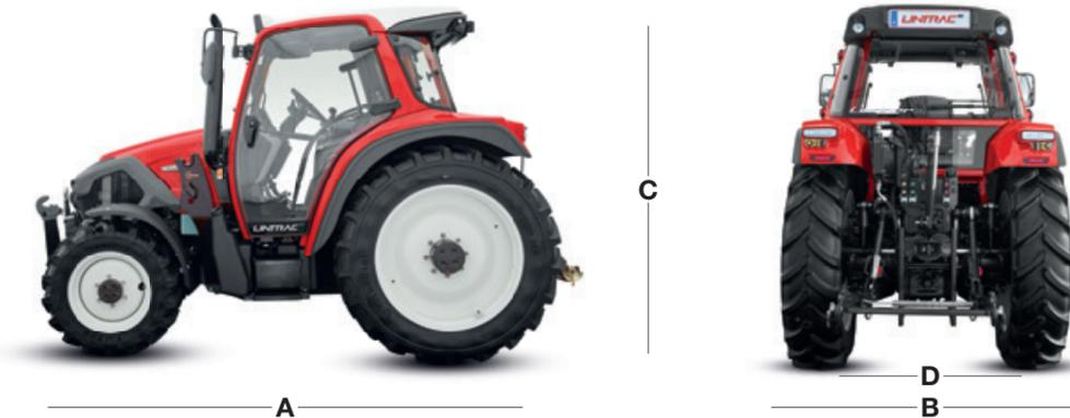
**Motor:** Perkins-Turbo, 102 PS / 420 Nm, 4-Zylinder/ 3.400 ccm,
